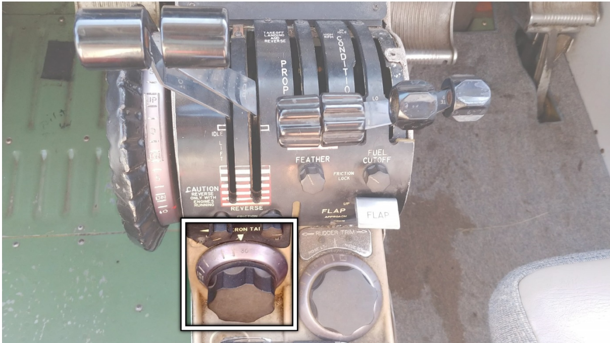
Figure 4. Aileron trim knob in its full left-wing-down position
