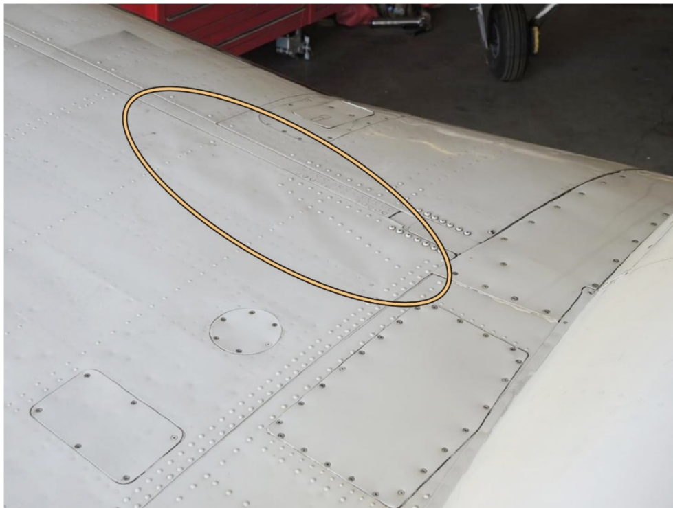
Figure 2. Wrinkles in the top skin of the left wing after the July 2016 accident
