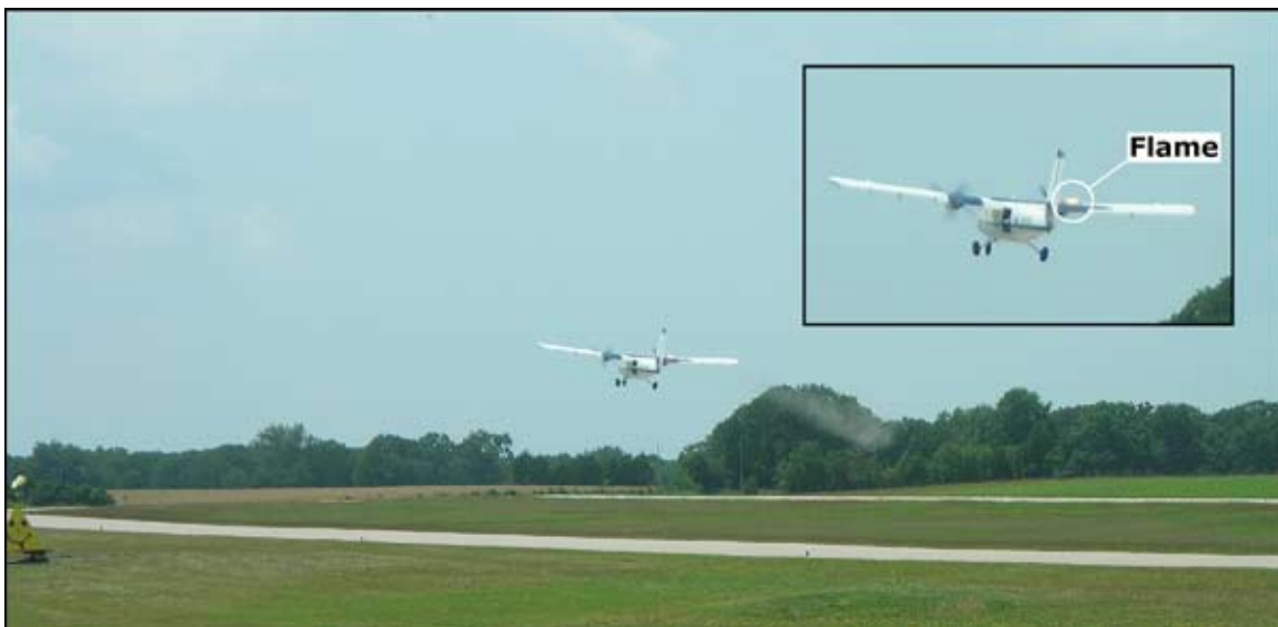
Figure 1. Witness' photograph showing accident airplane above the end of runway 24 with smoke and flames visible from right engine. (Inset shows an enlarged view.)
